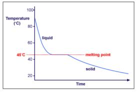
Okay the diagram above shows the cooling curve, how can we tell? The temperature is falling. The melting point is the same as freezing point, in this case its 45°C.
