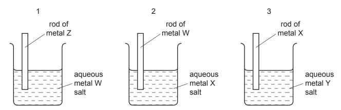
In beaker 1 metal W is displaced from solution.
