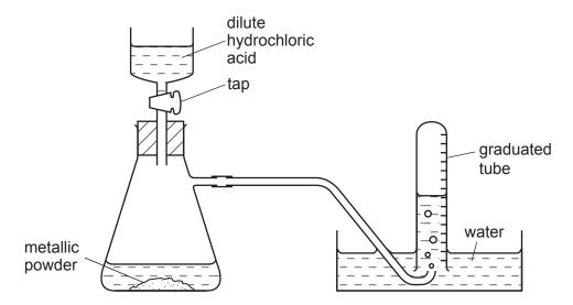
The experiment is carried out three times, using the same mass of powder each time but with different powders:
