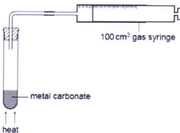
The student heats a 0.010 mol sample of each carbonate using the blue flame of the same Bunsen burner. She measures the time it takes for 100 cm<sup>3</sup> of gas to be collected in the gas syringe. The table shows her results.
