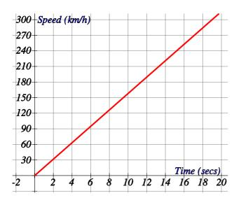
4) The speed-time graph below shows a old Mini accelerating. How fast is the car after 5 secs?
